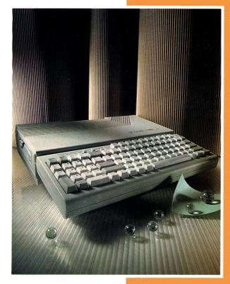
The Laser 128EX/2: faster than a GS in 8-bit mode, plus new internal 3½-inch drive, SmartPort, Control Panel, RAM card, and MIDI interface
