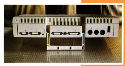
Laser 128EX/2 ports, left to right: joystick/mouse, parallel printer, MIDI/modem, video expansion, video out, external drive, MIDI/modem 2, serial printer, power plug, on/off switch.
