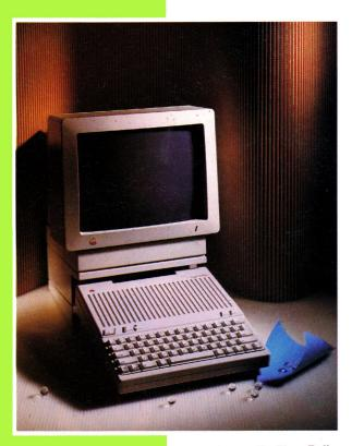
Apple's new IIc Plus: Builtin 312-inch disk drive, SmartPort, great speed, and an internal power supply bring an old favorite up to date.
