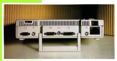
IIc Plus ports, left to right: joystick/mouse, modem, RGB video, composite video, SmartPort disk drive, printer, and powercable outlet.
